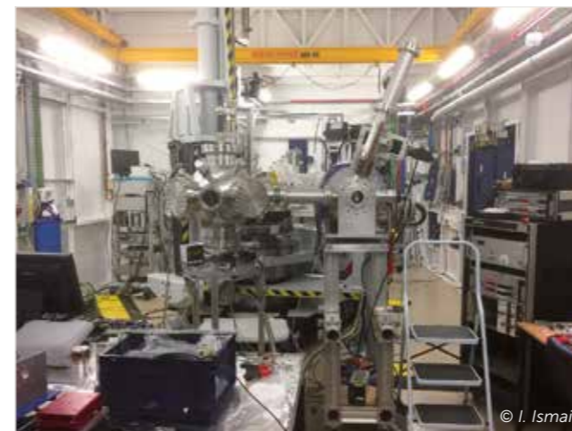
Figure 1: photograph of the one-crystal version of MOSARIX installed at GALAXIES beamline at SOLEIL Synchrotron.
