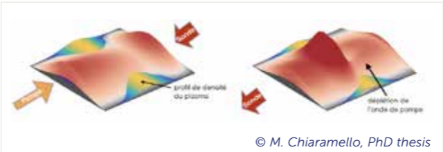
Figure 3: 2D simulations of a typical experimental situation showing the pump and seed crossing in the plasma at different times (5.8, 7.6 and 9.6 ps). The seed is amplified while the pump is depleted.
